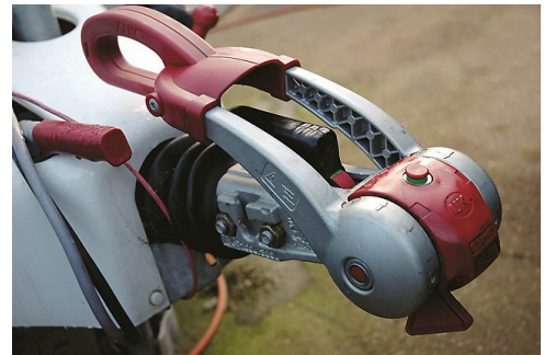
Often the head will have a coloured indicator to show when engagement is complete
